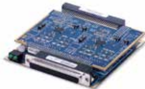
DNR-series boards such as this DNR-QUAD-604 are used with DNR-series RACKtangle chassis.
